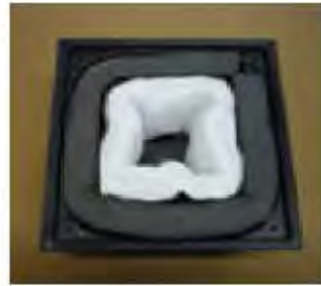
Fig.2 Install 3M foam and acoustic insulation.
