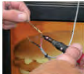
Fig.6 Solder all connections.
