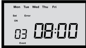
LEFT: Error displayed when trying to save Event 3. Adjust the ON / OFF times and try to save again.
